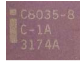
This is a pre-production Intel 8035 released at Step level C-1A
