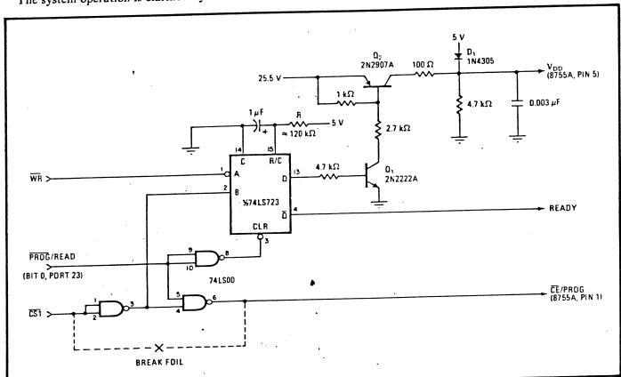
**Loading up.** Minimal hardware and small byte-transfer routine simplifies programming of E-PROMs in SDK-85 one-board microcomputer design kit. Given starting and ending addresses of RAM data to be transferred, low-cost package programs 1 byte of E-PROM on each pass, then checks for parity at termination of run. If run terminates prematurely, E-PROM location causing fault will be displayed in register BC.
